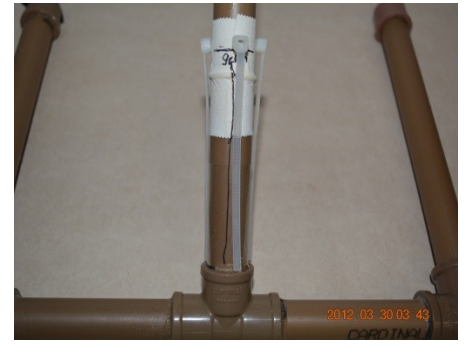
Fig. 15. Base com as 4 abraçadeiras de nylon.
